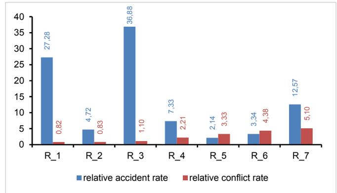
Fig. 5. Comparison of relative traffic accident rates and relative traffic conflict rates  $k_R$  on 7 roundabouts
